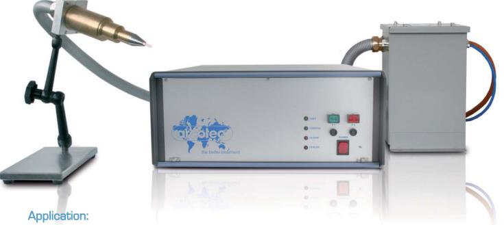
The Arcospot® PGS 061 device is used for the in-line pre-treatment of moulded parts, profiles, adhesion grooves and folded boxes. Treatment speeds exceeding 200m/min. can be achieved. The treatment clearance from the surface is approx. 6-10mm.
